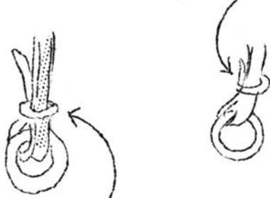
METHOD OF ATTACHING STRAPS TO RINGS
