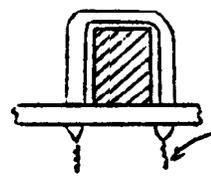
Cross section of spring at axle. Notch spring to hold axle.
